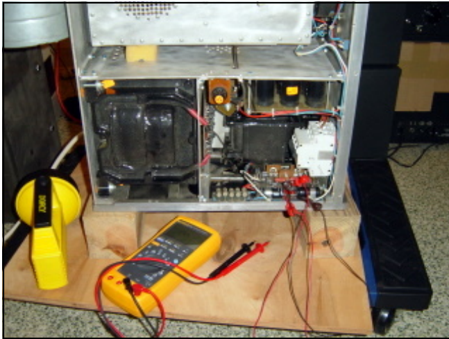
Careful Ed, even a bad plate supply can be DANGEROUS. Pull that fuse and find and check the caps before debugging
